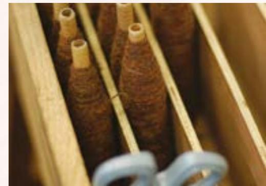
The Barleycorn uses an irregular loom set up, so a new set of shafts was prepared with the yarn rethreaded for the particular draft sequence. Large cones of the wheat coloured warp yarn are split into smaller 'cheeses' (cylindrical yarn packages as opposed to conical ones), for loading the creel to make the warp.
